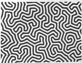
Fig. 1: Remnant state with equal areas of each domain. Magnetising field 0.00 H sat
